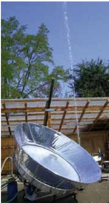
The solar water pump „Sunpulse“ meets these requirements as a sustainable means. Sunpulse pumps water from storage lakes or ground water of up to 60 metres deep thus ensuring the irrigation of an average family business. As energy source it simply needs the sun – which is not only protecting the environment but also saving operational expenses.
